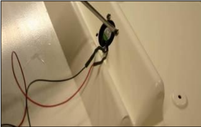
Figure 14a: Evaporator fans
